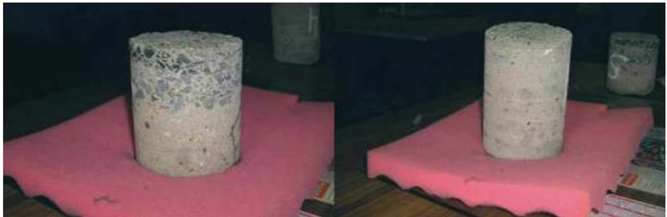
Fig. 5: A core of cement-sand mix with a concrete wearing course
