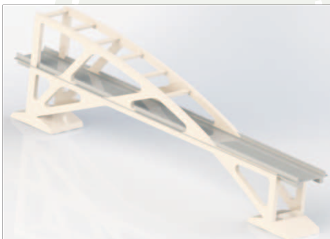
Fig 1: Proposed 65m span bridge across Gori nadi
