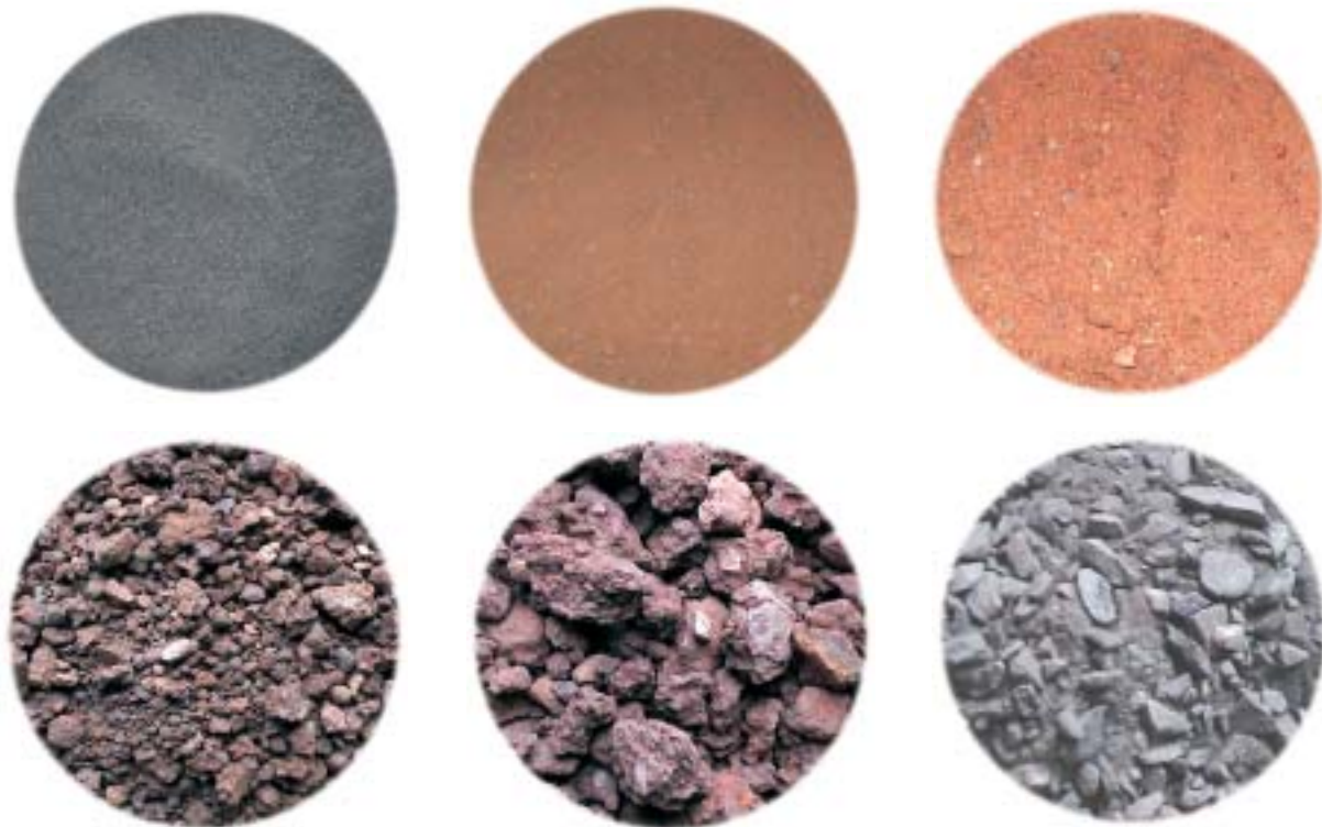
FIG. 2 : VISUAL CLASSIFICATION OF SOILS AND GRAVELS (TOP-LEFT TO RIGHT) CLAY, SILT AND SAND. (BOTTOM-LEFT TO RIGHT) MOORUM WITH EXCESSIVE FINES, MOORUM AND GRAVEL
