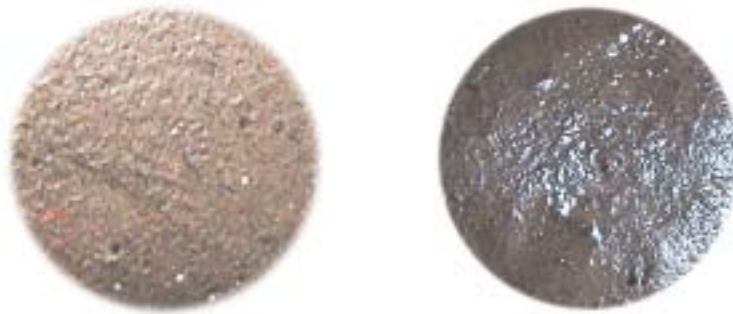
FIG. 3 : DILATANCY TEST FOR SILTY SOILS
