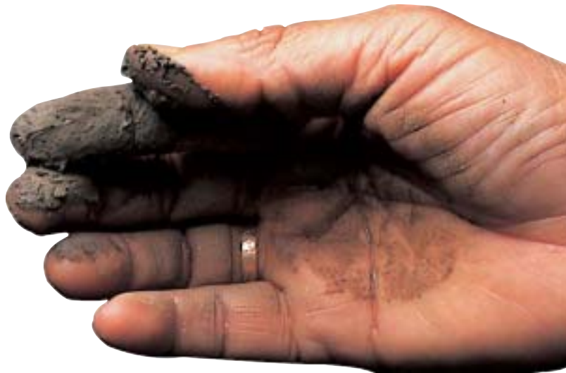
FIG. 4 : HAND-FEEL 'STAIN' METHOD FOR TESTING CLAYEY SOILS
