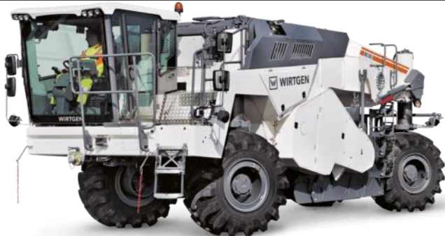
Recycler – WR240 (2.4m width)
