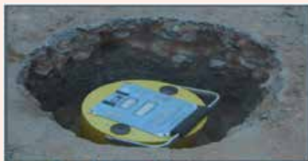
a Acquiring elastic moduli using geogauge
