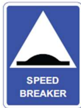
Fig. 17.48 Speed Breaker Informatory Sign
