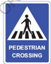
Fig. 17.47 Pedestrian Crossing Informatory Sign
