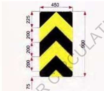
Fig. 15.78 Two Way Hazard Marker
