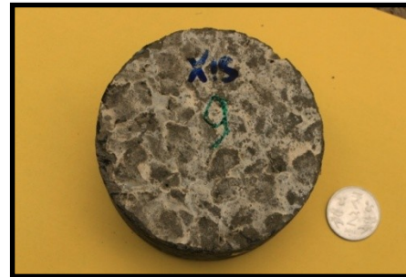
Top surface (Core taken from Pavement)
