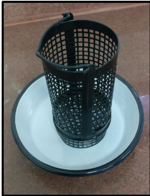
Drain Down Apparatus
