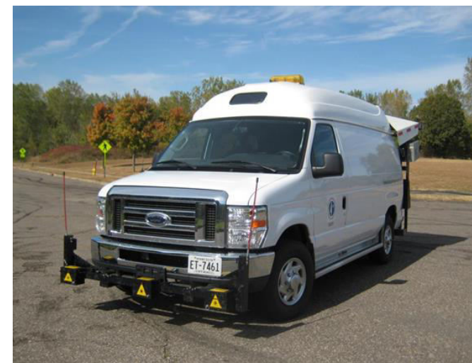
MnDOT's Pathway Services, Inc. Digital Inspection Vehicle (DIV)
