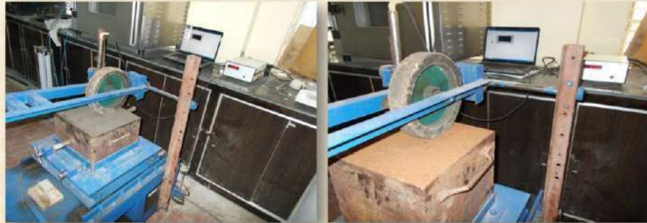
Experimental setup with 300 x300 x 200mm fabricated mould
