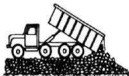
3 Back Dump Aggregate
