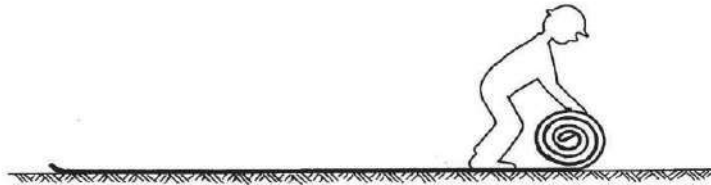
B. Unroll the geotextile directly over the ground to be stabilized. If more than one roll is required, overlap the rolls. Inspect the geotextile and pull it out tight. Stake down as needed.
