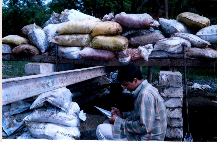
Plate 3.4 Recording the values of Pressure and Deformation
