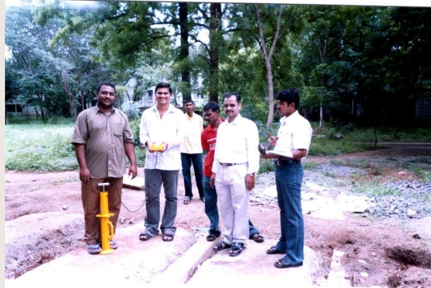
Plate 3.5 Recording the Instant CBR value using Clegg Impact tester
