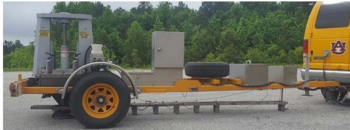
Figure 1.1 – Dynatest Model 8000 FWD.
