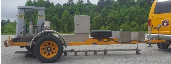
Figure 1.1 – Dynatest Model 8000 FWD.
