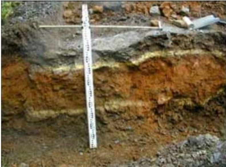
A test pit taken in a low volume road exhibiting rutting
