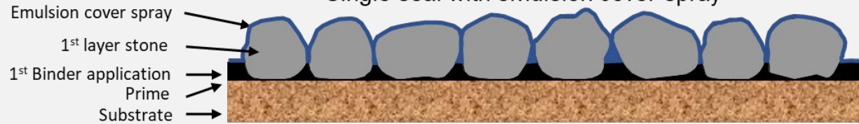
Single seal with emulsion cover spray
