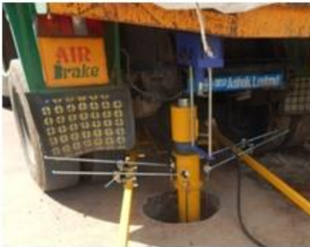
Static Load Plate Test
