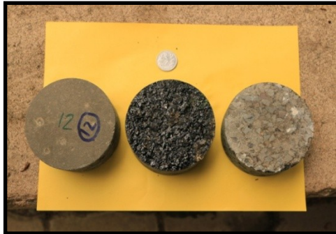
Middle Core shows the bottom of CGBM Layer Surface
