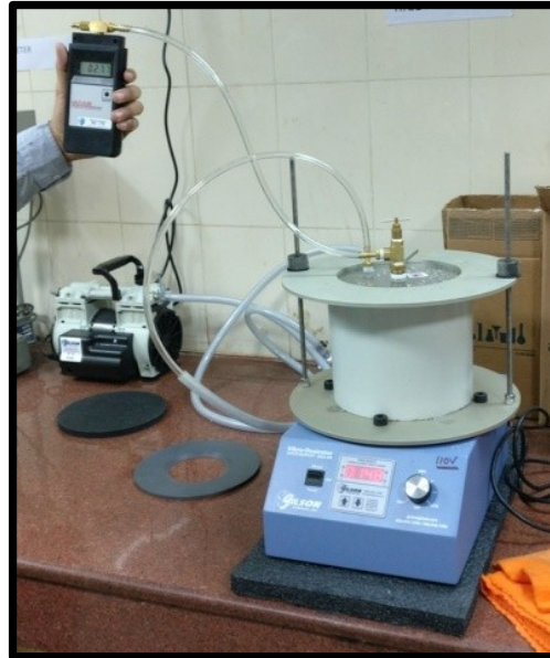
Rice Apparatus for calculating Theoretical Maximum Specific Gravity ( G_{mm} )
