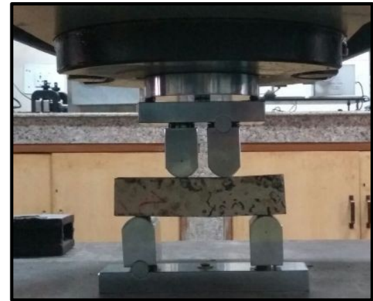
Modulus of Rupture Test Set up in UTM
