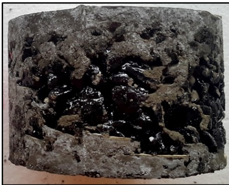
Partial Depth of grouting
