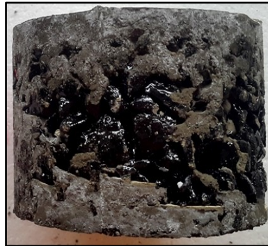
Partial Depth of grouting
