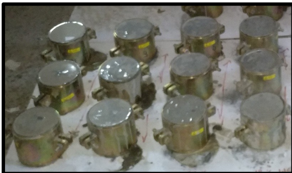
Grouted Bituminous Mix in Split Mould
