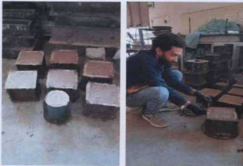
Fig.11. Cube molds for determining UCS and durability tests.
