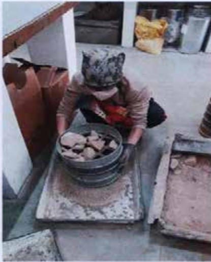
Fig. 4 Removing oversize aggregates.
