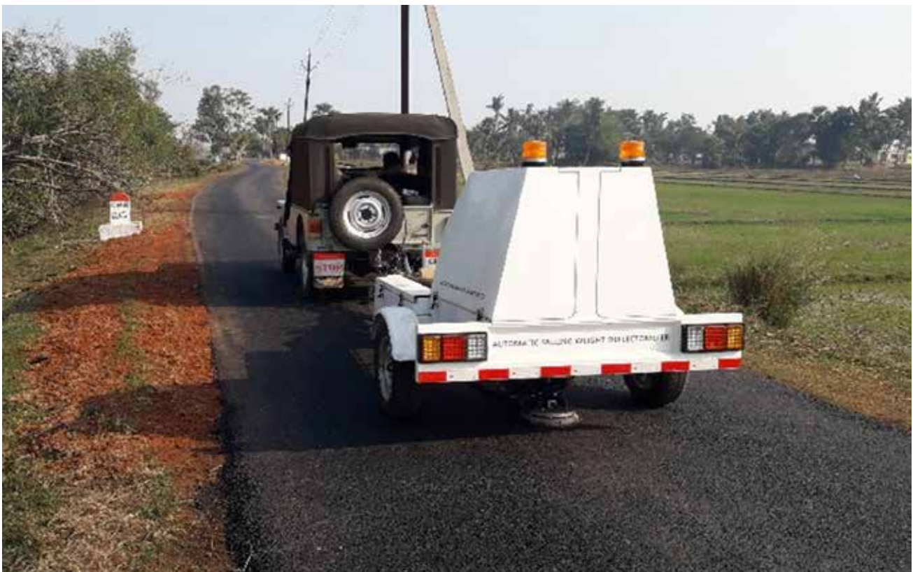
FIGURE 14: Structural Evaluation using FWD
