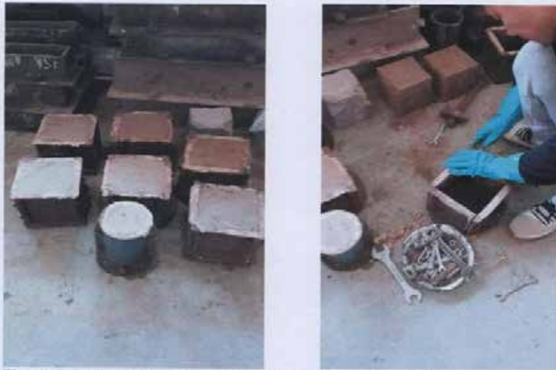
Fig.10. Cube molds for determining UCS and durability tests.
