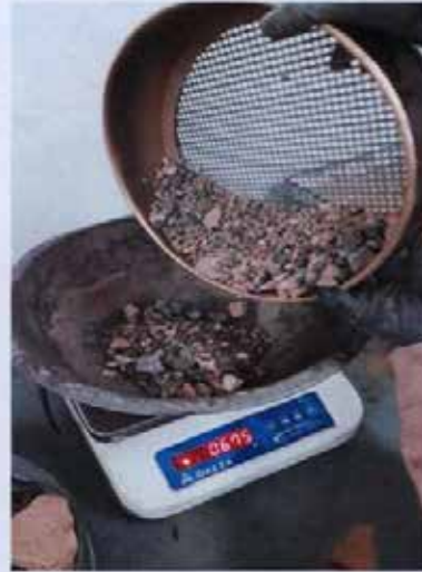
Fig.5 Weighing sieved materials.
