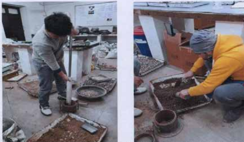
Fig.3 Preparation of cylindrical molds for determining optimum moisture content & maximum dry density.
