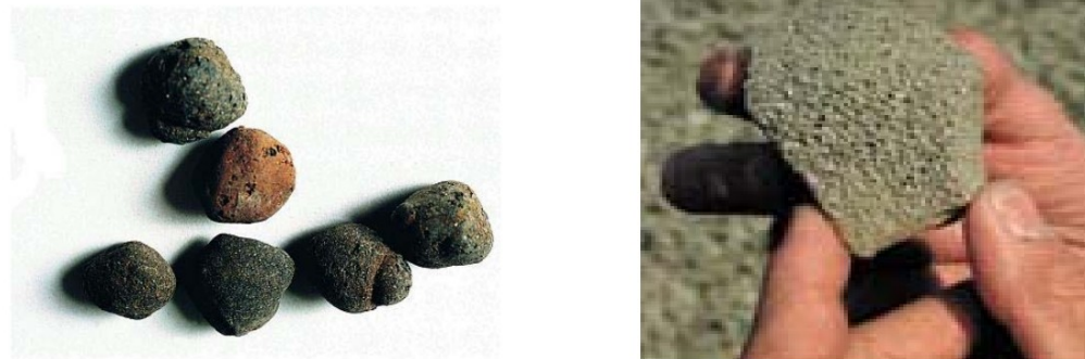
Figure 1 – Leca LWA to the left, Hasopor foam glass aggregate to the right
